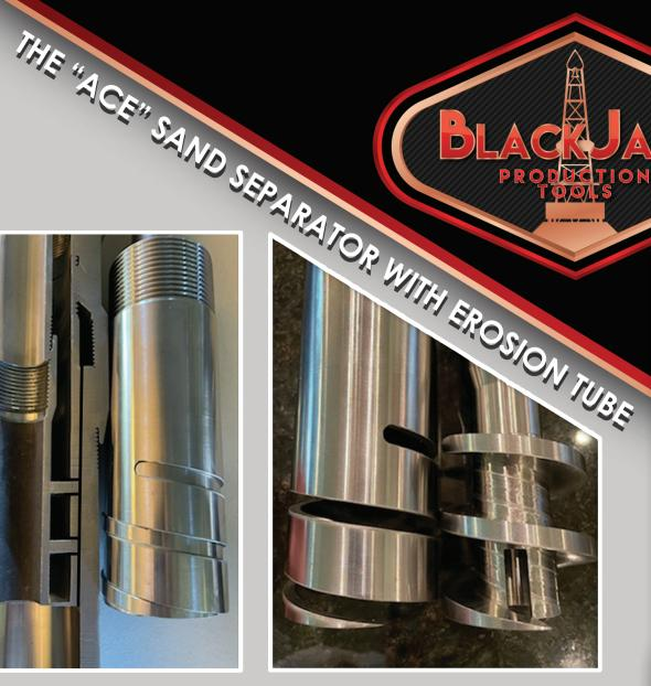
The "ACE" Sand Separator with Erosion Tube is a safer, longer-lasting sand separator. The fully-machined sand spiral is sheathed first by a hard barrel with a matching spiral cut, so the blades thread into that which we call the "erosion tube," then we sheath that with an even heavier tube.
